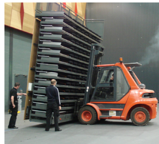
Type M - Mobile. Once closed, units can be specified to be moved via (pictured left to right): a pair of hydraulic trucks, hydraulic trucks with an additional power truck to assist, fork lift truck, or air hover system.
