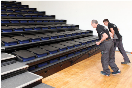
Manual operation via removable pull handles.
